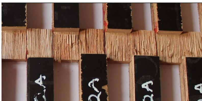
Fig. 3: Tested shear samples showing above 80% wood failure.
