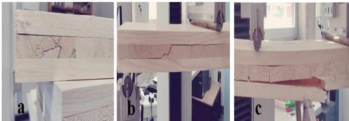
Fig. 9: Bending failure in aspen CLT [a] delamination, [b] rolling shear and [c] tension failure.
