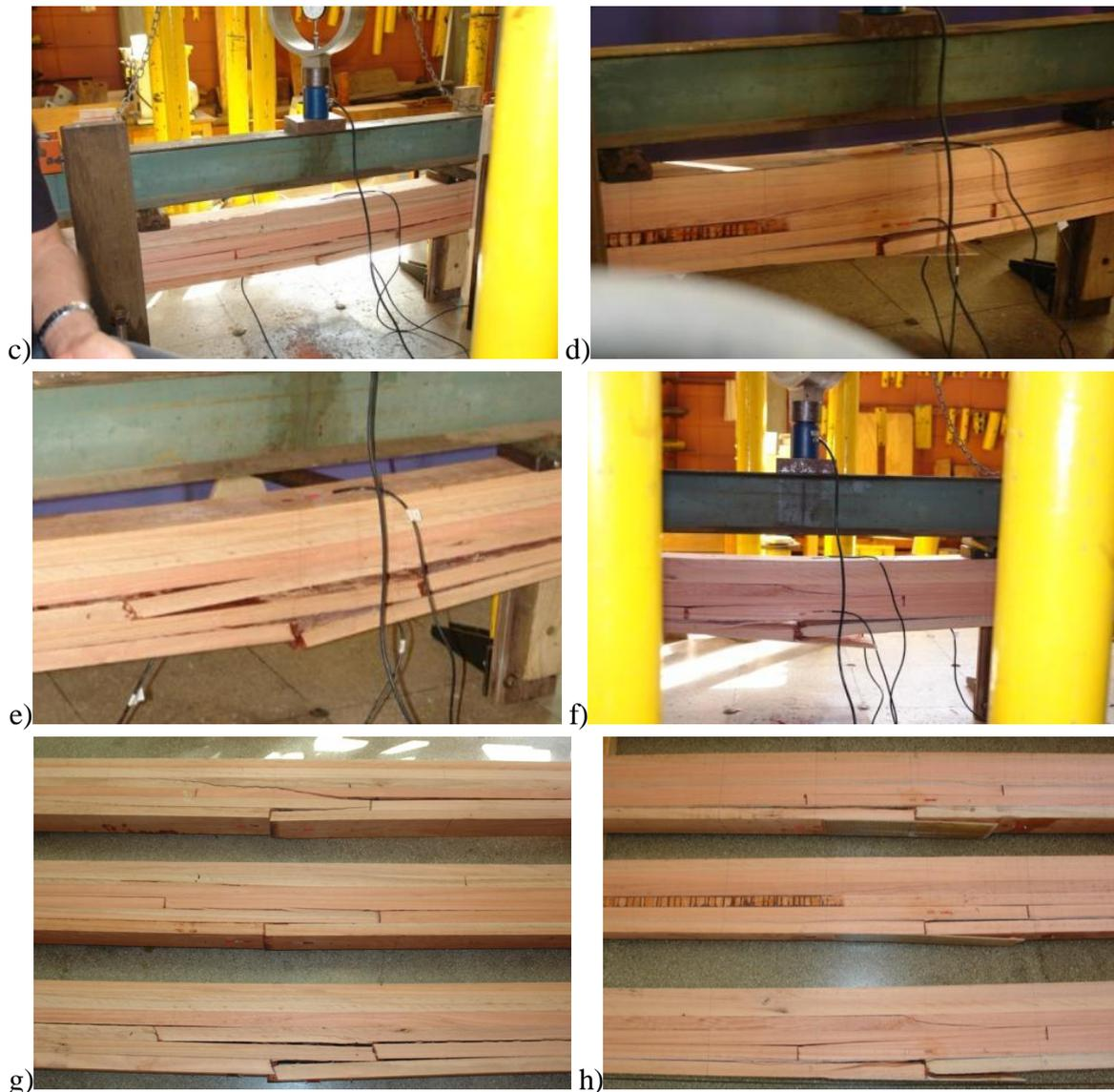
*Fig. 3: Failure of glulam: a) unreinforced beam 1; b) reinforced beam 4; c) unreinforced beam 2; d) reinforced beam 5; e) unreinforced beam 3; f) reinforced beam 6; g) unreinforced beams 1, 2 and 3; h) reinforced beams 4, 5 and 6.*
