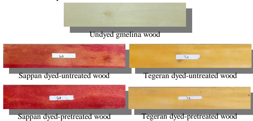
Fig. 4: The appearance of uncolored and colored gmelina wood using sappan and tegeran. Sample size of 20 cm in length, 5 cm in width, and 2 cm in thick.
