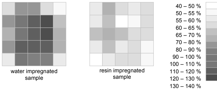
Fig. 3: MC of cross-section samples after freeze-drying of 24 hours. The MC of resin impregnated sample is based on the dry wood plus solid content of resin
