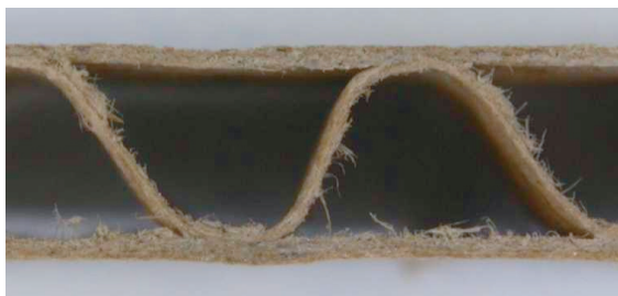
Fig. 1: Cross section of corrugated board before a pressure test
