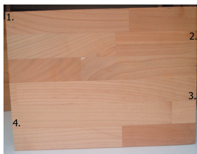
Fig. 1: The sample of cherrywood board with dimension parts for colour measurement
