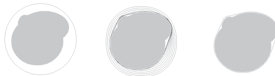
Fig. 1: Active Contour, a) Initial Contour, b) Contour Evolution c) Final Contour
