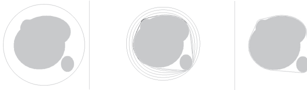
Fig. 2: Active Contour and distraction points, a) Initial Contour, b) Contour Evolution, c) Final Contour
