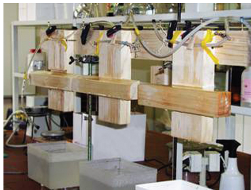
Fig. 3: Experimental system of artificial wetting
