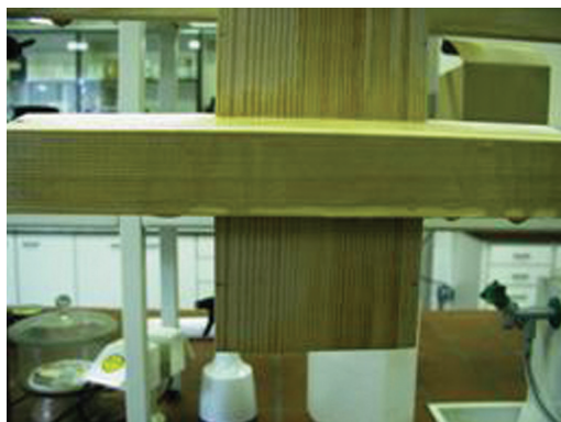
Fig. 8: Water mass retained on edges
