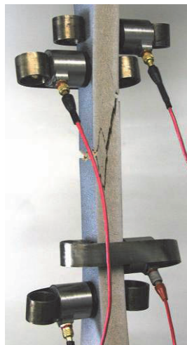
Fig. 4: Position of the 4 sensors for the acoustic emission analysis
