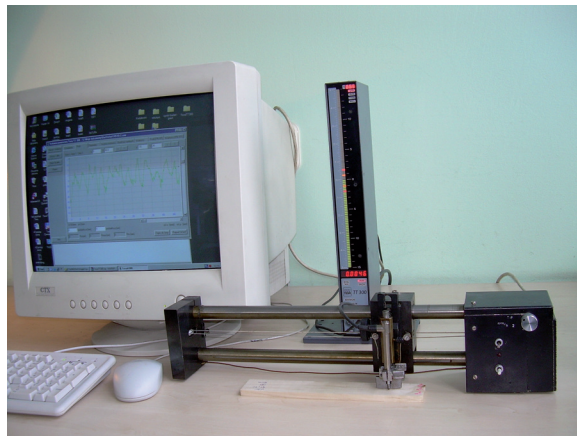
Fig. 1: The device on measurement of surface roughness
