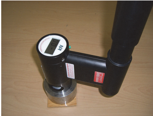
Fig. 1: Determination of adhesion strength with a standard test device
