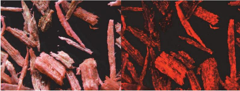
*Fig. 2: Blended beech particles fraction 0,600 (magnification 20×)*
