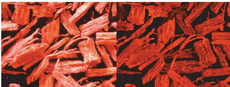
*Fig.5: Blended beech particles fraction 1,500 (magnification 20×)*
