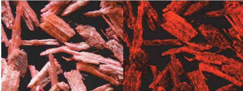
*Fig.3: Blended beech particles fraction 1,000 (magnification 20×)*
