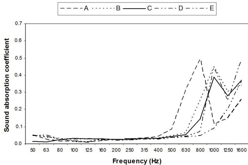
Fig. 4: Sound absorption properties determined for different surface drilling percentages: A= 0.8 %; B= 1.4 %; C= 1.8 %; D= 2.1 %; E= 4.0 %
