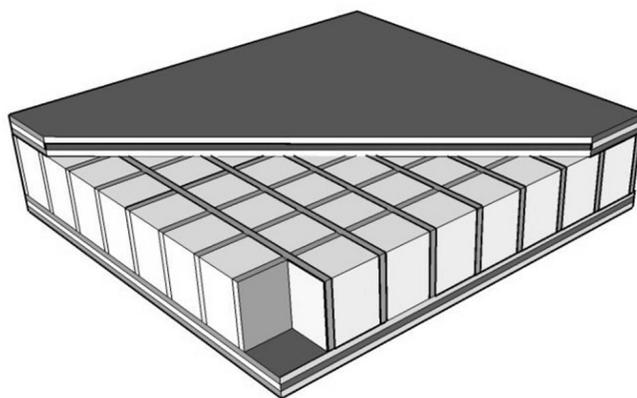
*Fig. 3 : Illustration of the commercial sandwich panel*
