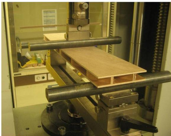
Fig. 2: Bending strength test performed on the wood-based composite
