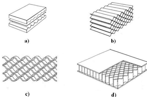
Fig. 1: Scheme of the production process of the lightweight panel
