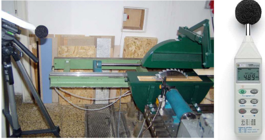
Fig. 6: Chauvin Arnoux noise meter and its placing at the experimental stand.
