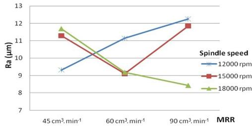
Fig. 6: The influence of spindle speed and MRR on surface roughness.
