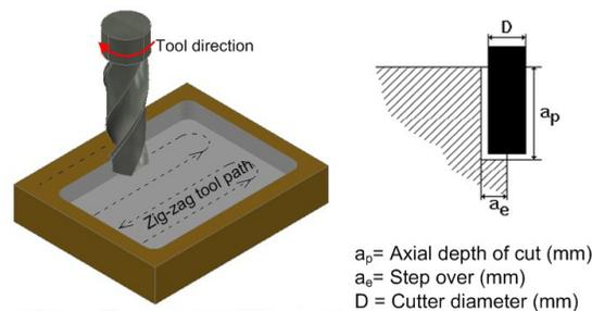
Fig. 2: Parameters of pocket milling surface.
