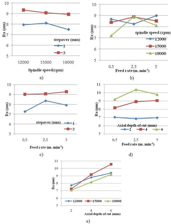
Fig. 5: The effect of dual interactions processing parameters on Ra, a) the interactions of spindle speed\* stepover b) the interactions of feed rate\* spindle speed c) the interactions of feed rate\* stepover d) the interactions of feed rate\* axial depth of cut e) the interactions of axial depth of cut \* spindle speed.
