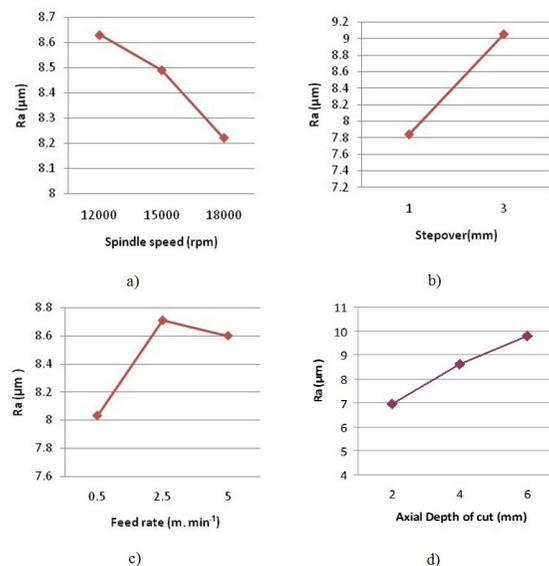
Fig. 4: The effect of processing parameters on surface roughness (Ra).
