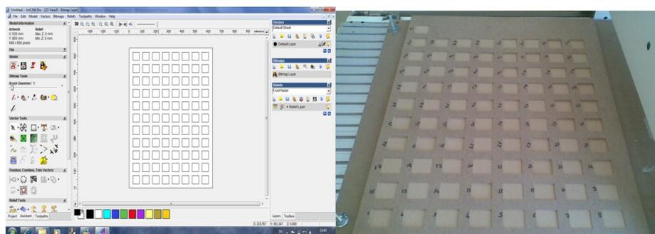
Fig. 3: CAD/CAM design and machined on MDF panels.
