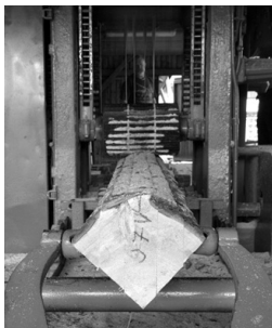
Fig. 5: Processing of quarter logs into radial planks Fig. 6: Storing of radial planks in the sawmill. of 60 mm.
