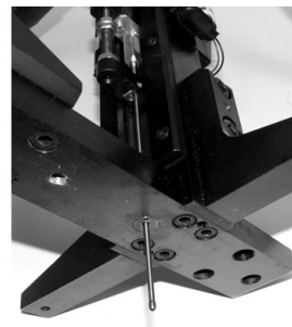
Fig. 2: Detail of pin passage through the tool base.
