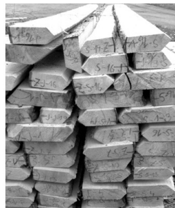
Fig. 5: Processing of quarter logs into radial planks Fig. 6: Storing of radial planks in the sawmill. of 60 mm.
