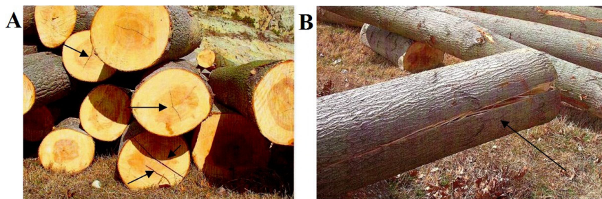
Fig. 1: Appearance of cracks on cross sections of poplar logs (see arrows) after tree felling and bucking A. In B, an intensive crack extended along the log.
