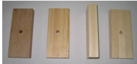
Fig. 1: Embedment test series: Oak - solid timber (OK), Pine - solid timber (PN), Spruce -vertical glulam (SP-V), Spruce - horizontal glulam (SP-H).
