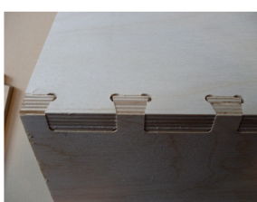
Fig. 1a (left) and 1b (right): The produced dovetail joint (left) and the description of the joint parts – the tails and the pins (right). Fig. 2: Typical progress of the shape of router bit edge wear.
