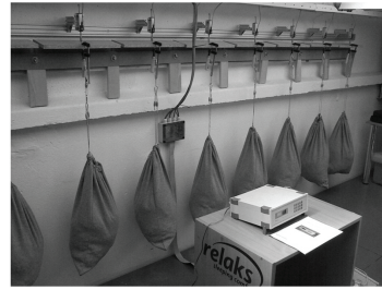
Fig. 5: Diagram of the experimental stand. Fig. 6: Measuring station for calculating joints reliability. Source: Own elaboration
