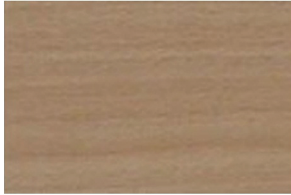
Fig. 2: Surface of seasoned and milled beech sapwood after thermal treatment using saturated water steam with temperature of t = 125\text{--}130^\circ\text{C} for the duration of \tau = 6.5 h.
