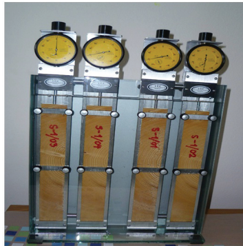
Fig. 1: Specimens inserted into the Swellometer instruments.
