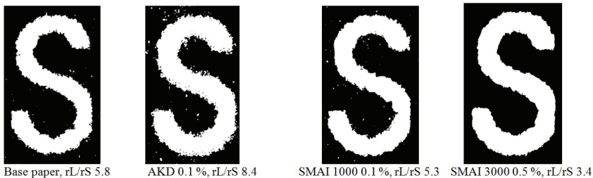
Fig. 3a: The thresholded image of yellow dye letter on black background of base paper and modelled papers.
