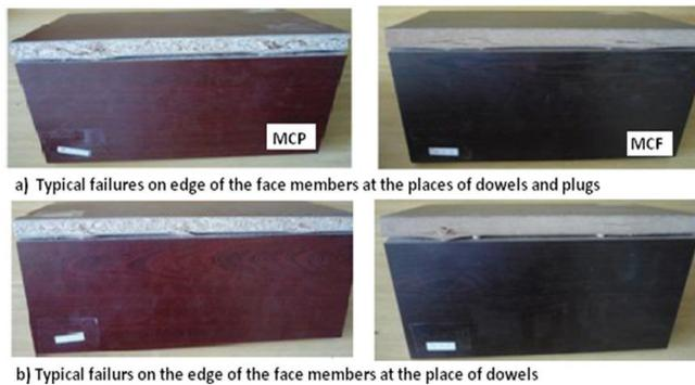
Fig. 7: Typical failures on the edges of face members.
