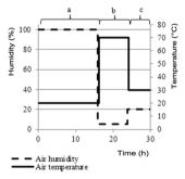
Fig. 2: Changes in humidity and temperature during full one cycle of weathering: a) soaking in water for 16 hours, b) drying at 70° C for 8 h, c) UV irradiation for 6 hours.
