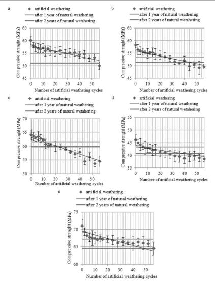
Fig. 1: Statement of results testing mechanical properties of wood during artificial and natural weathering: a) – heartwood of Scots pine, b) – sapwood of Scots pine, c) – garapa, d) – European oak, e) – angelim pedra.
