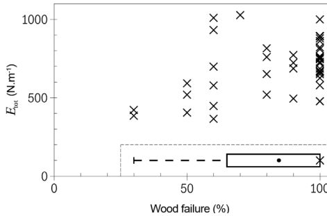
Fig. 6: WFP of PRF bonded specimens. The black dot in the boxplot indicates the mean value and the cross indicates the median.
