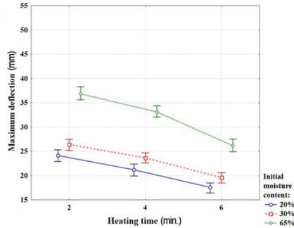
Fig. 5: 95 % confidence interval shows the influence of heating time and initial moisture content on maximum deflection.
