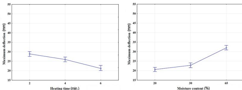
Fig. 4: 95 % confidence interval shows the influence of heating time (left) and initial moisture content (right) on maximum deflection.
