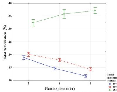
Fig. 3: 95 % confidence interval shows the influence of heating time and initial moisture content on total deformation.
