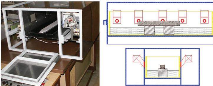
Fig. 1: Microwave device, an overview (left), side view (up right) and front view (bottom right) (Gašparík and Barčík 2013).
