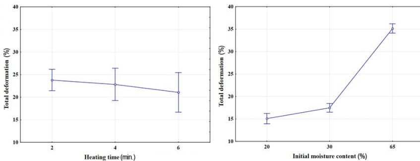
Fig. 2: 95 % confidence interval shows the influence of heating time (left) and initial moisture content (right) on total deformation.
