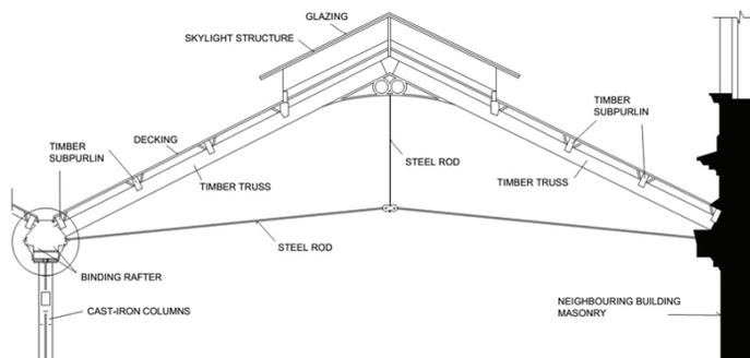
Fig. 6: Scheme of a vestibule roof structure of the Masaryk Railway Station in Prague.
