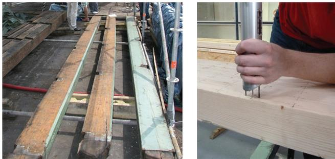
Fig. 2: a) situation on site during in-situ investigation, b) Pilodyn measurement.
