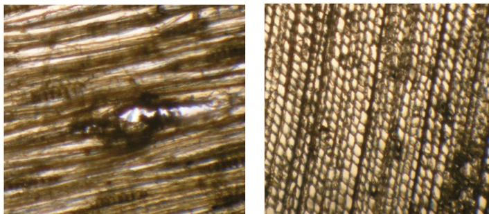
Fig. 4: Wood anatomy of the investigated structural elements; a) detail of a resin canal of spruce (*Picea*), b) cross section of fir (*Abies*), © ITAM AS CR.
