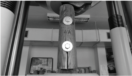
Fig. 6: The failure of statically tested samples in the press EU100.
