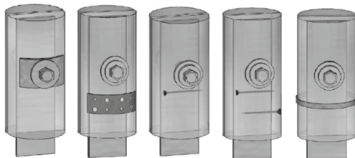
Fig. 3: Half – models of reinforced samples.
