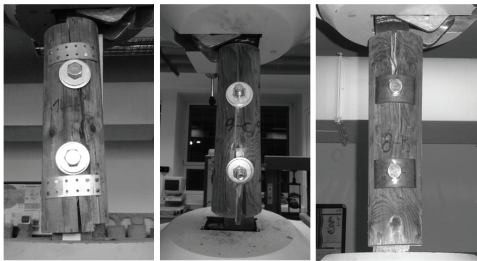
Fig. 11: Failures of reinforced joints with BOVA plates (left), one screw (middle) and modified washers (right).
