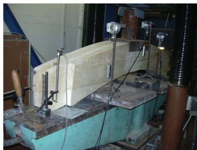
Fig. 13: View of the experimental test of curved segments.
