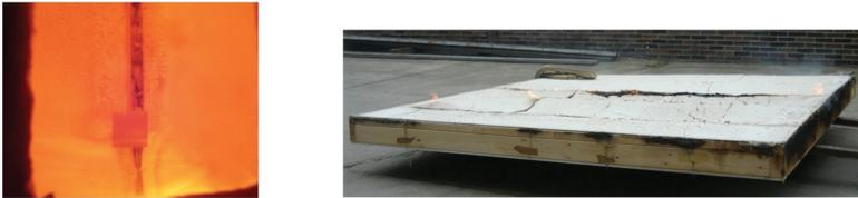
Fig. 5: The furnace in 65<sup>th</sup> minute (left) and the wall assembly after the fire test (right).
