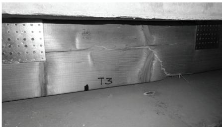
Fig. 11: Damage of timber beam in knot.
