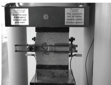
Fig. 9: Concrete sample test for getting elastic modulus of tension and compression.
