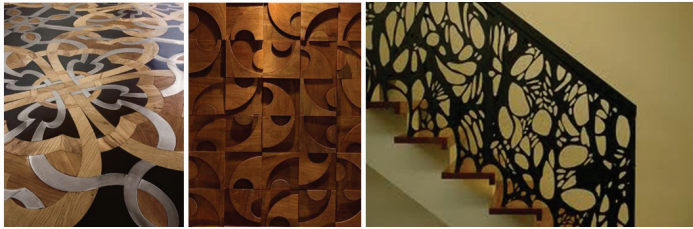
Fig. 1: AWJ use alternatives for the structural joinery items fabrication: a) wooden floors, b) walls facing and c) stairway handrails.
