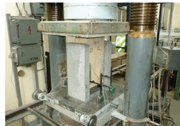
Fig. 3: The testing machine with a push-out specimen.
