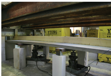
Fig. 6: The Four-point bending test configuration of a composite timber concrete T-beam.
