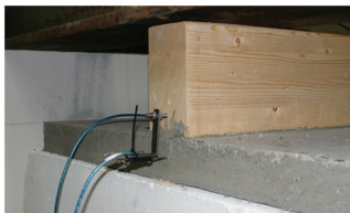
Fig. 16: Slip horizontal movement measuring.
