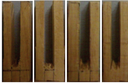
Fig. 6: Prong test of the dried rubberwood from different width size of the sample: a) 25.4 mm b) 50.8 mm c) 76.2 mm d) 101.6 mm.
