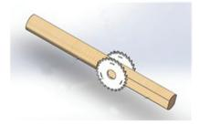
Fig. 2: Diagram of bilateral trimming saw.
