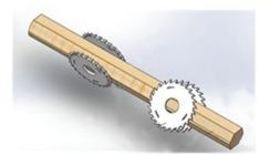
Fig. 3: Diagram of four-sides sawing.
