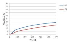
Fig. 3: Course of weight loss for wood of low (LD2) and high (HD2) density treated with a double layer of fire retardant.
