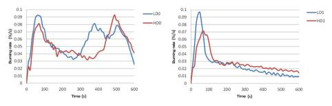
Fig. 5: Course of burning rate for unrefined wood of low (LD0) and high (HD0) density.
