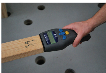
Fig. 2: Measurement of sample by device timber grader.
