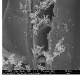
d) Collected PM with small size by wood rays (3000 $\times$ )
