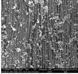
a) The adsorbed PM onto the surface (100 $\times$ ,
