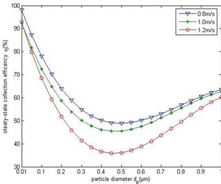
Fig. 8: The effect of permeate flow rate on steady-state collection efficiency of pits ( $T=453.15\text{ K}$ ,  $h=6\ \mu\text{m}$ ,  $\varepsilon=92\%$ ,  $d_{pore}=20\ \mu\text{m}$ ).
