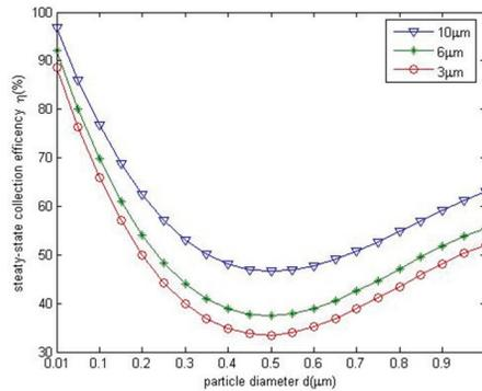
Fig. 10: The effect of tracheid wall thickness on steady-state collection efficiency of pits ( $T=453.15\text{ K}$ ,  $U_{wx}=1.0\text{ m}\cdot\text{s}^{-1}$ ,  $\varepsilon=92\%$ ,  $d_{\text{pore}}=20\text{ }\mu\text{m}$ ).
