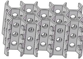
c) 3D model of micron wood fiber cell structure
