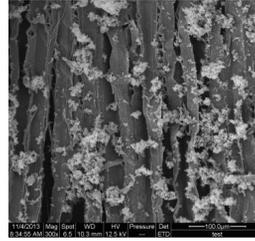
b) The adsorbed PM is onto the surface (300 $\times$ )
