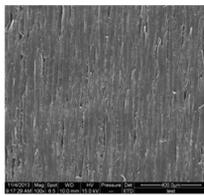
a) The deformed tracheids by external force (100×)
