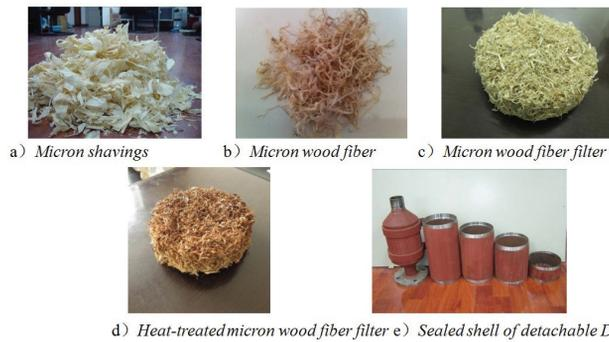
Fig. 1: Manufacturing Process of heat-treated micron wood fiber DPF.
