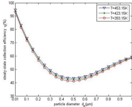
Fig. 9: The effect of exhaust temperature on steady-state collection efficiency of pits ( $U_{wx}=1.0\ \text{m}\cdot\text{s}^{-1}$ ,  $h=6\ \mu\text{m}$ ,  $\varepsilon=92\%$ ,  $d_{pore}=20\ \mu\text{m}$ ).
