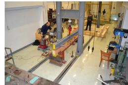
Fig. 5: Loading assembly under the STN EN 408. Fig. 6: Loading assembly.
