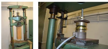
Fig. 1: Universal hydraulic testing machine with a specimen (left), force transducer and inductive deformation sensor (right).
