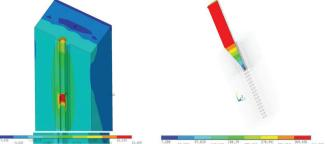
Fig. 5: Tension Sx and von Mises stress for the force F=76.40 kN.
