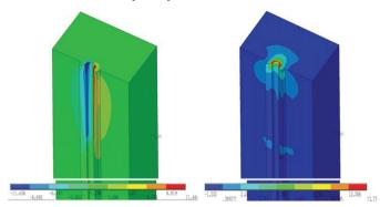
Fig. 6: Shear Sxy and tension Sy stress for the force F=76.40 kN.
