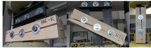
Fig. 9: Damaged squared timber samples in tension at different angles.
