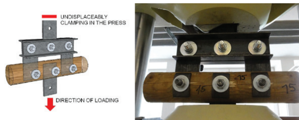
Fig. 1: Steel product for testing in tension perpendicular to the grain and sample in the press machine.
