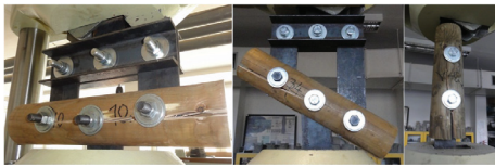
Fig. 8: Damaged round timber samples in tension at different angles.
