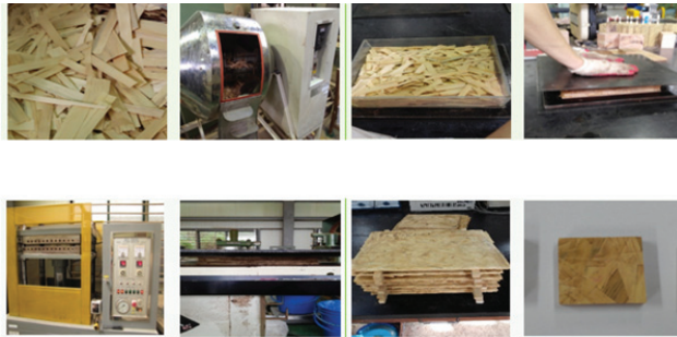
Fig. 1: Production line of flakeboards at the laboratory.
