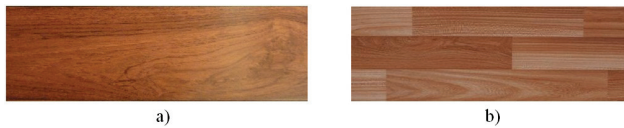
Fig. 2: The two types of decorative veneers: a) mono-block and b) three splice.
