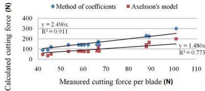
Fig. 6: The ratio between measured and calculated values of cutting force for both models.
