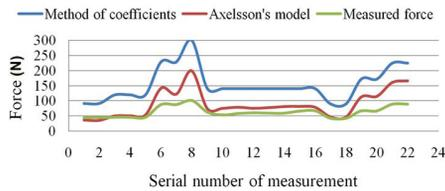
Fig. 5: Measured and calculated mean cutting forces in peripheral milling of oak.
