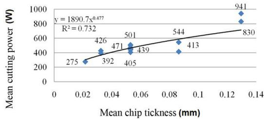
Fig. 2: The dependence of the measured cutting power and mean chip thickness in peripheral milling.
