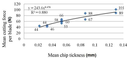
Fig. 4: The dependence of mean cutting forces per cutter blade and mean chip thickness in peripheral milling.
