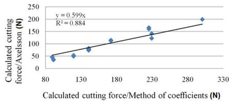
Fig. 7: The ratio between values of cutting force calculated by coefficient methods and Axelsson's models.
