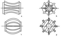
Fig.2: Schematic structure of upward (a b) and downward(c d) arc milling cutters.
