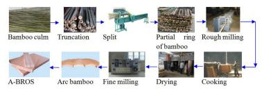
Fig.1: Process of arc bamboo manufacture in practice.
