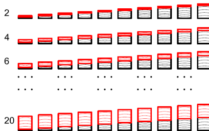
Fig. 3. Hard material with constant thickness placed on the upper side of layered material.
