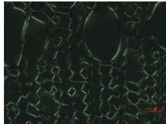
d. The layers of early wood and late wood.
