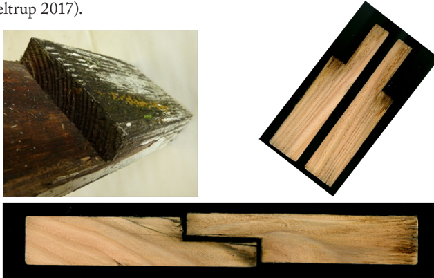
Fig. 6: Douglas fir specimens after 20 years of exposure. Top left: Opened lap-joint and fruiting bodies of Dacrymyces spp. on the upper surface. Top right: Interior brown rot decay starting from the lap-joint. Bottom: Douglas fir lap-joint with brown rot decay starting from the end grain.
